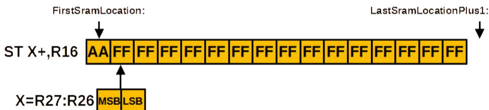
The first step has been executed, **ST** has written the content of register R16 to the first SRAM location. The plus behind X auto-increases the address right after writing the register to the location in X. It replaces two instructions:
