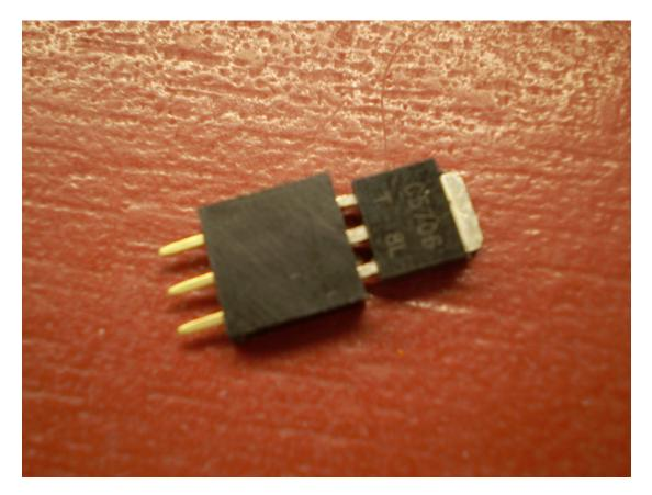
Figure 158: PA transistor socket
