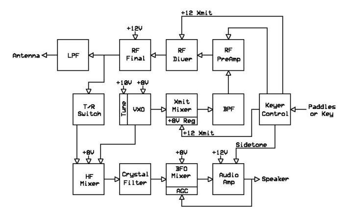
Figure 2: 1W block diagram.
