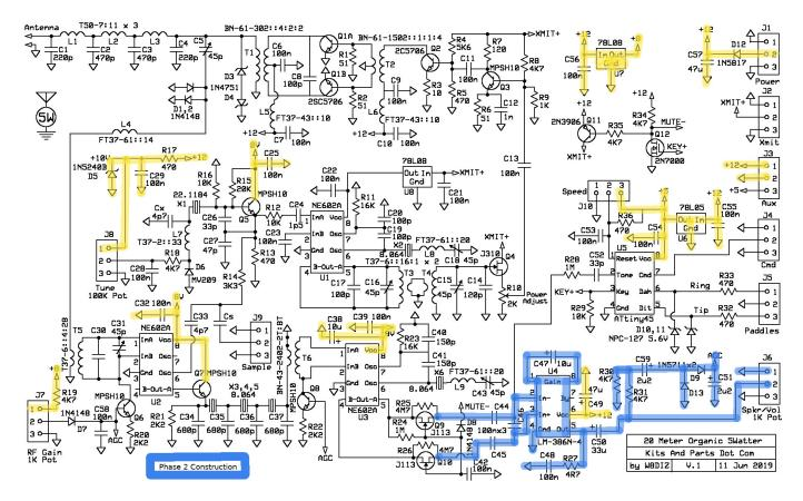
Figure 7: Phase 2 installation in blue.
