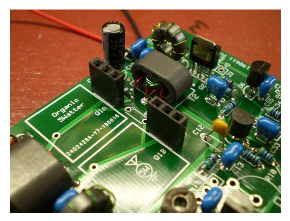
Figure 159: Q1A and Q1B sockets
