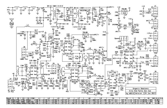
Figure 168: Schematic of 5W Transceiver.
