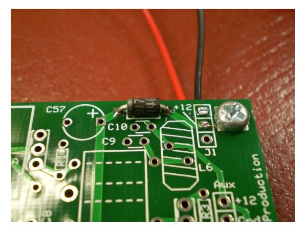
Figure 12: Power supply wires and D12.
