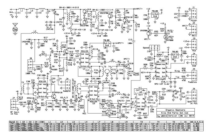
Figure 4: 5W schematic version 1.
