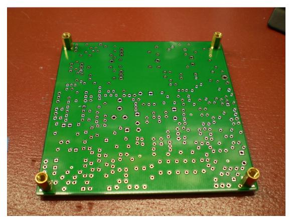
Figure 11: Bottom view showing brass standoffs.
