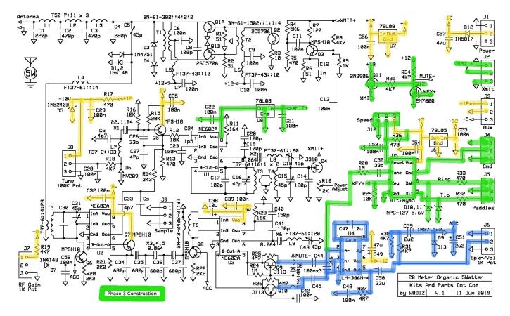
Figure 8: Phase 3 installation in green.
