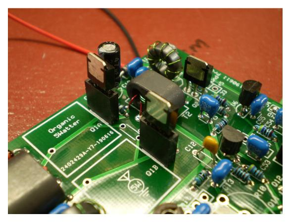
Figure 160: Q1A and Q1B transistors
