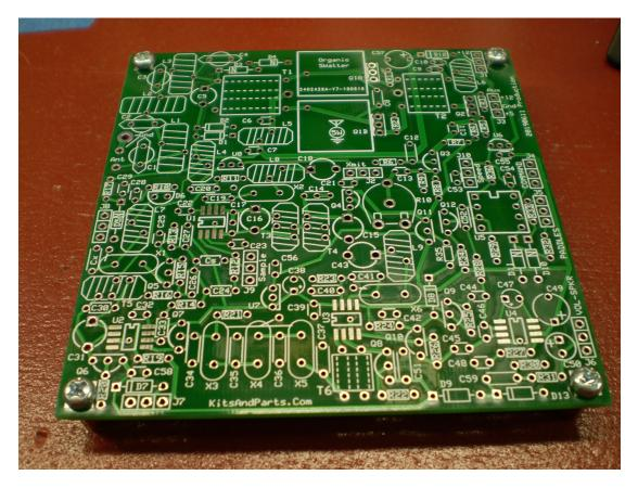
Figure 10: Standoffs mounted on the corners.
