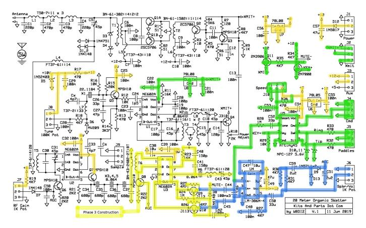
Figure 9: Phase 4 installation in yellow.
