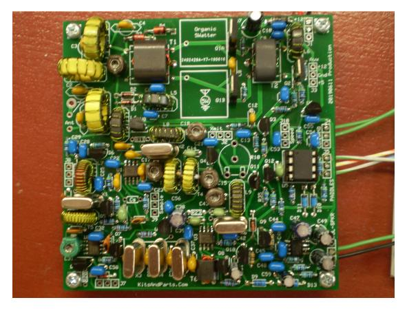
Figure 162: Assembled Transceiver Board
